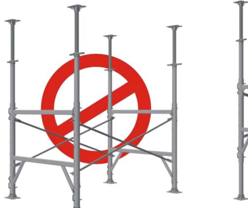
BAD SET-UP(s) (UNBALANCED), FOR USE WHERE THE TOWER SITS ON LEVEL CONCRETE AND REQUIRES EXTENSION AT ONE END.
