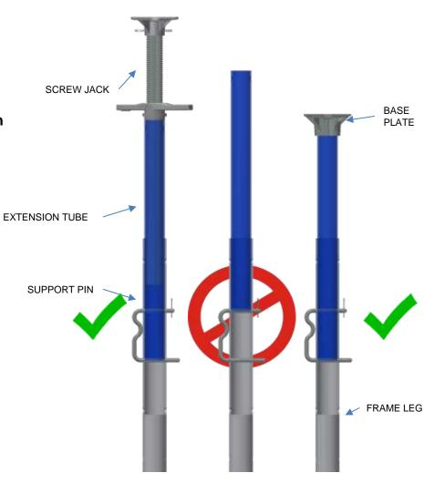
ALWAYS ENSURE THAT U-PIN IS PROPERLY ENGAGED INTO BOTH THE FULL AND ½ HOLE OF THE EXTENSION TUBE TO PROVIDE EQUAL DISTRIBUTION OF LOAD BEARING ON THE U-PIN AND FRAME LEG.
