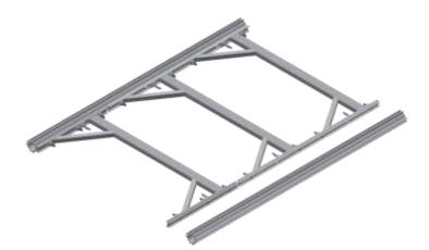
1. Set up a level work area to assemble the frame legs and ledgers.
