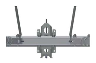
WEDGE UNIT SHOULD BE LOCATED EXACTLY IN THE CENTRE POSITION – WHERE DIAGONAL STRUT MEETS.
